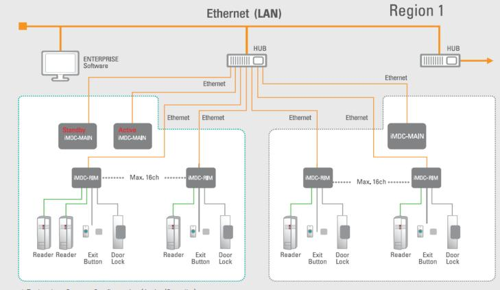
\* Redundant System Configuration (Active/Standby)
