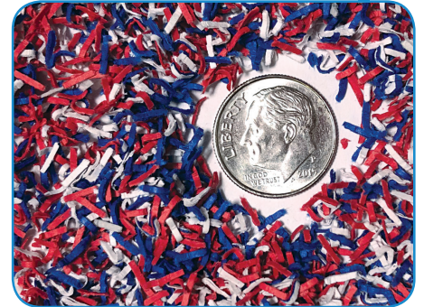
Paper media shredded particles are 0.8mm x 4.5mm in size
