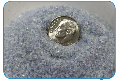
Optical media particles are <math>1.5\text{mm}^2</math>, nearly as fine as salt
